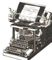
A Burroughs Billing Machine. One of the many kinds of adding, bookkeeping, calculating and billing machines built by the Burroughs Adding Machine Company.
